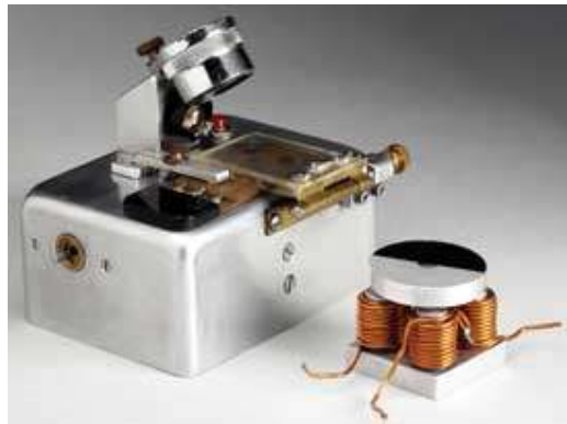
In 1960, William McLellan used his lunch breaks to build a micromotor (0.5mm long), winning $1000
